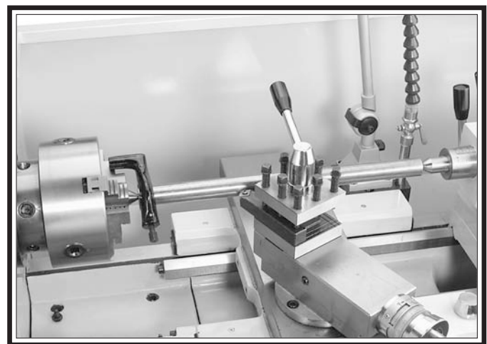
Figure 60. Example photo of a workpiece mounted between the centers.
